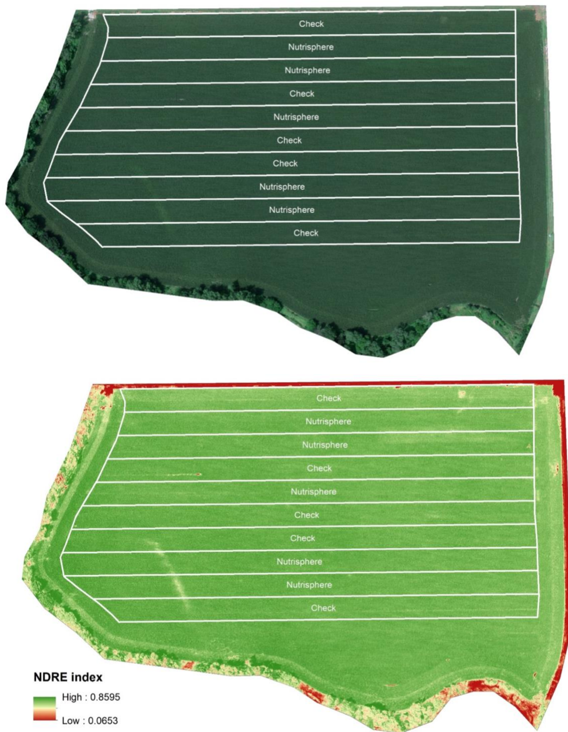
Figure 1. True color imagery (top) and normalized difference red edge index (NDRE) from August 2, 2018.
