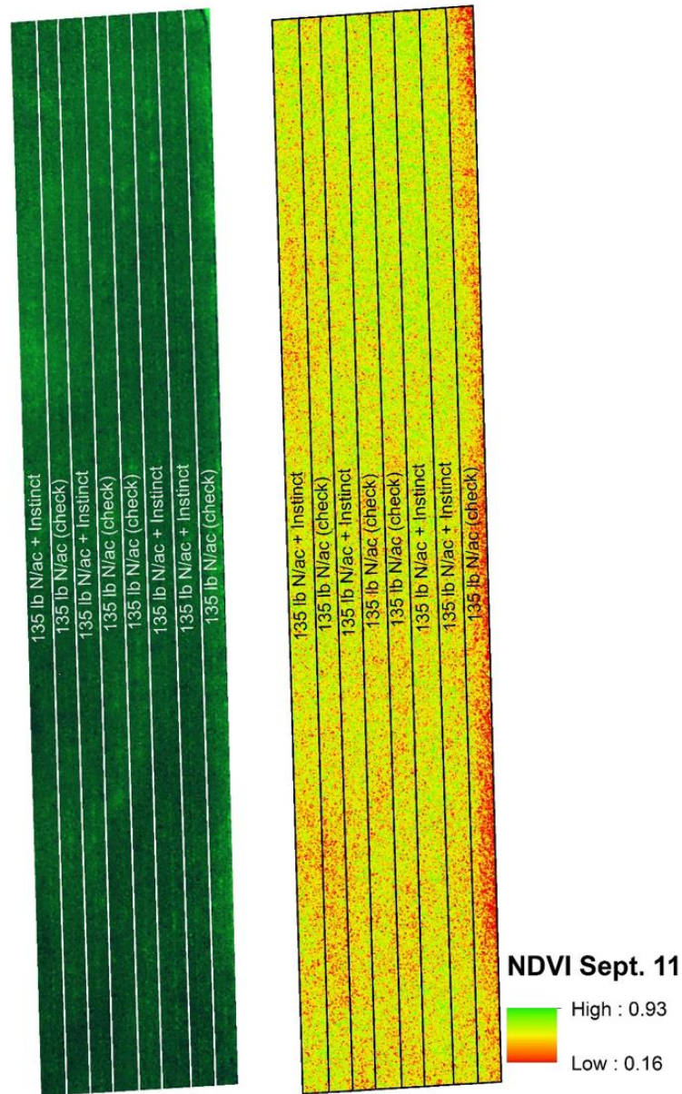
Figure 1. True color (red-green-blue) imagery (left) and NDVI (right) from September 11, 2017.
