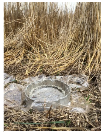
Figure 2. Soil water infiltration test conducted following wheat harvest.
