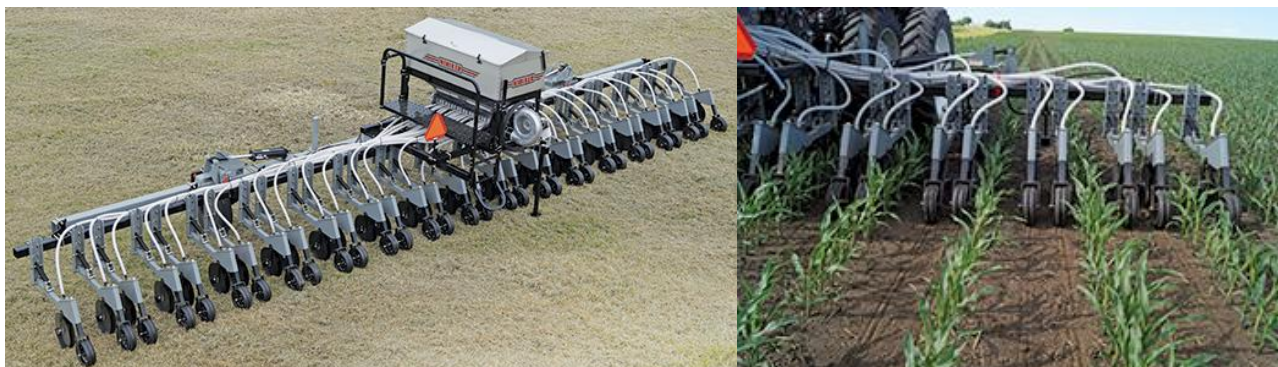
Figure 1. Hiniker twin row interseeder used to establish cover crops. Images from Hiniker ( https://www.hiniker.com/ag_products%20new/sp_cover-crop-seeders.html ).
